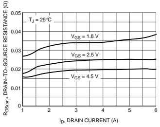
Figure 3. On-Resistance versus Drain Current
