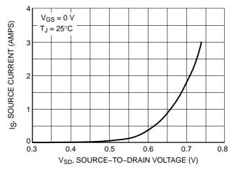
Figure 10. Diode Forward Voltage versus Current
